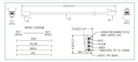
Look at the cable ends in the pic to the right and you'll see the wires are the same by color, pin 1 to 1, pin 2 to 2, etc. on each connector.
