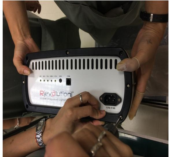
**Fourth,** remove the six screws that hold the heatsink in place on top. There are two (2) hanging eyes and four (4) machine screws.
