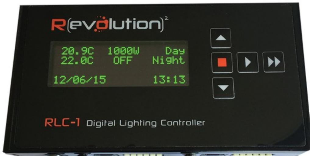
Congratulations on your new all-digital lighting controller! The RLC1 can control up to 512 lights in two zones with up to 256 lights in each zone. The RLC1 can control any Revolution or compatible light such as the Phantom, MaxiBright, etc.
