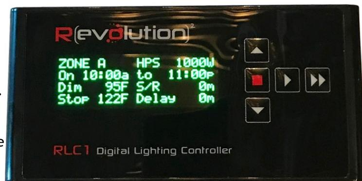
You can also set the Delay function to delay the lights coming back on after a power outage. The RLC1 has an internal clock and starts counting when the power goes out so a 30 minute on-delay will only have 10 minutes to run if the power comes back on in 20 minutes. This minimizes change to your photoperiod.
