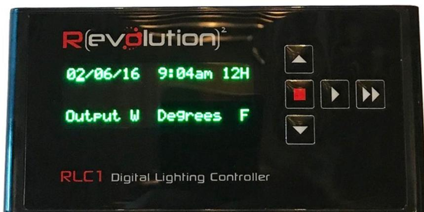
3. Press the **Page** button until you bring up Zone A to set up your first room. Each Zone page lets you choose the type of light you have and the size ballast driving it. A 1000w HPS like the DEva has six (6) power settings while a 315w CMH has two.
