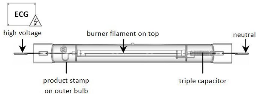
**Usage** The lamp must be ignited at specified ignition voltage and operated at rated lamp power (+/- 3%)
